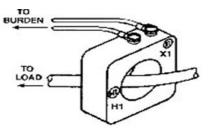
CT's are generally located in the main breaker panel or in branch distribution panels where space is always at a premium. CT's do not have to be installed 90 degrees to the conductor run they are generally held in place with plastic tie wraps. CT's with mounting feet are available if appearance is important and there is enough room to accommodate this type of mounting arrangement.
