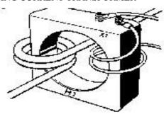
A "Selection Guide" is provided in this catalog to aid in selecting the type of CT for your application. Non-standard ratios can be obtained by looping the conductor through the window to add or subtract current flow.
