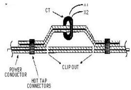
Window type CT's should be mounted with the H1 side of the window towards the power source. The X1 secondary terminal is the polarity terminal. The polarity marks of a current
